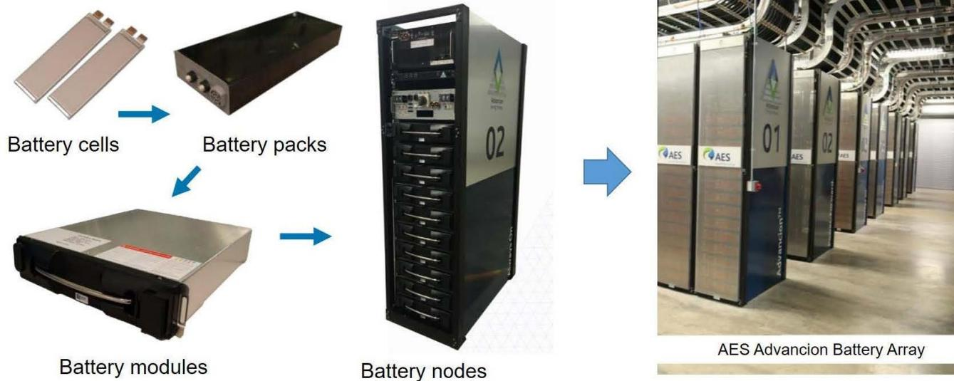
Assembly principle of single battery cells into larger scale storage units. Source: AES Energy Storage
