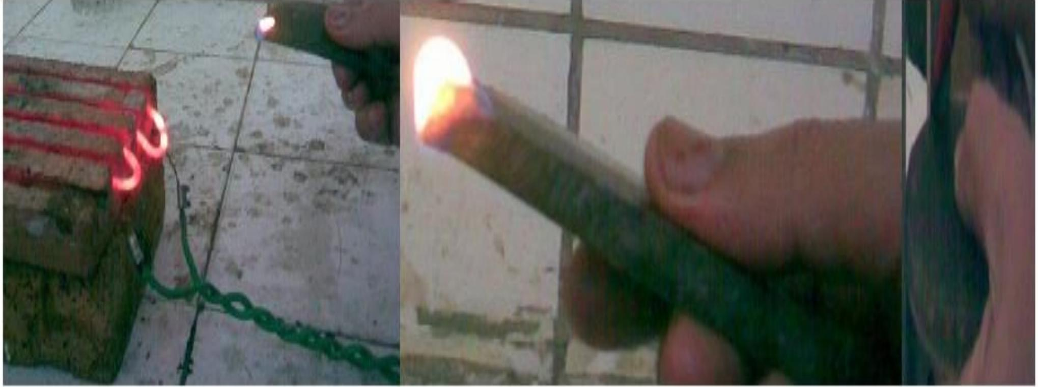
Figure 11. Fire resistance test up to 100°C
